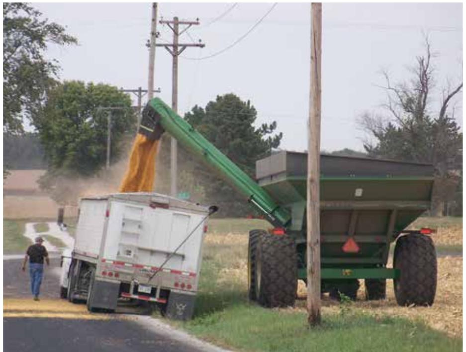
large machinery near power lines. Do not let the spotter touch the machinery while it is being moved anywhere near power lines.
